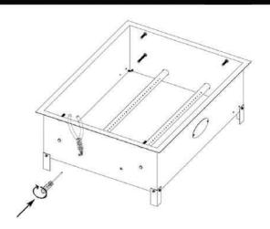
Step 1 -Fix the gas burners by tightening the screw, holding the nut through sharp nose plier.
