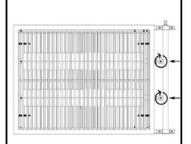
Step 1 - Make sure the gas valves are fully closed. (Clockwise)
