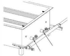
Step 5 - Release the washer valve away from the burner for more air intake, hence less carbon emission. (Flame Colour - Light Blue)
