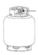
Step 3 - Connect the regulator to gas cylinder and switch on. (Rotate Clockwise) [Conventional Low Pressure Gas Regulator is Recommended]
