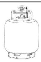
Step 9 - Remove the gas regulator from the Gas Cylinder.
