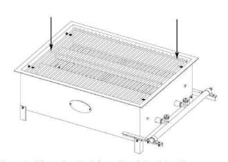
Step 6 - Place the Stainless Steel Cooking Grates on top of the grill.
