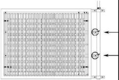
Step 8 - Once charcoal is lit or Gas grilling is finished, Turn off the gas valve fully. (Rotate Clockwise)
