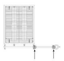
Step 2 - Insert the hose in gas inlet and regulator and tighten the hose clips on both sides.
