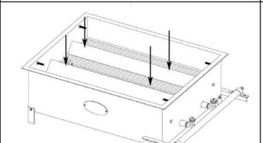
Step 5 - Place the Stainless Steel Heat Shield on top of the charcoal grates covering the burner.
