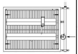
Step 4 - For Gas grilling, start the lighter, point towards the burner (Under SS Heat Shield)and open the gas valve slowly to ignite the burner.(Anticlockwise)
