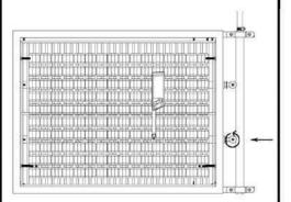
Step 7 - Start the lighter, point towards the burner and open the gas valve (anticlockwise) to ignite the burner. Charcoal will be lit by this method.
