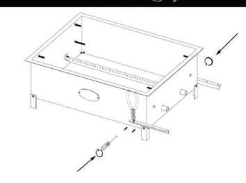
Step 2 - Fix the brackets through 2 screws on each side.
