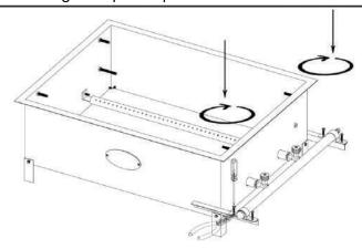
Step 3 - Fix the gas clip through 2 screws on each side.
